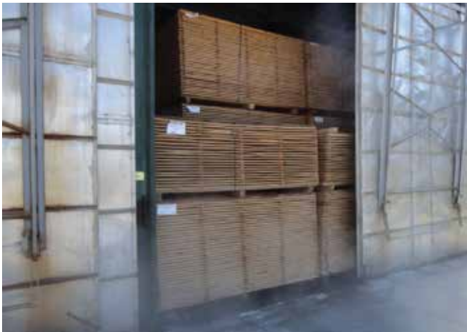
Kilns are used for drying lumber and plywood after treating. Carefully removing water from the wood results in consistent, high-quality FRTW.
